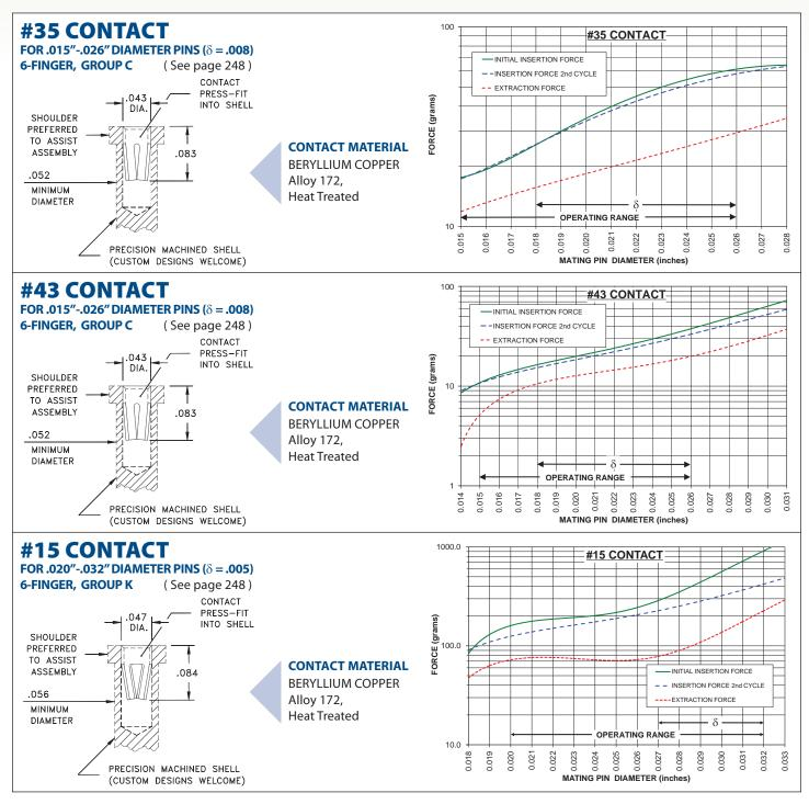
**The insertion / extraction force characteristics above** were derived using a 30 microinch gold-plated contact and polished steel gauge pins having a bullet-shaped tip.
