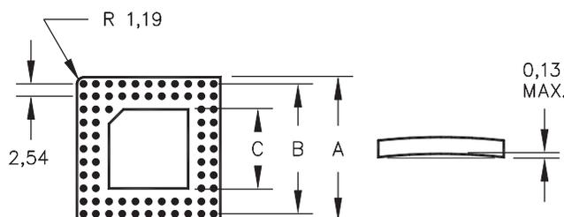
DIMENSIONS A, B, and C can be calculated as follows:
