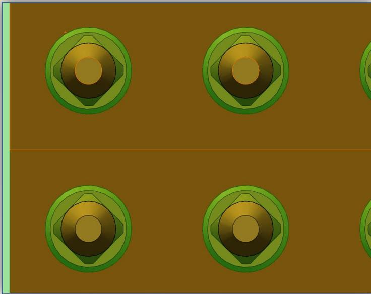
*View of 4994 compliant barrel from bottom side of PCB .*
