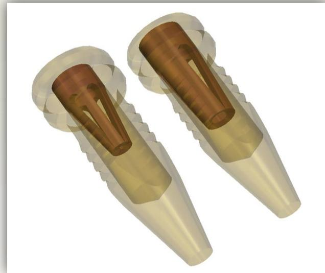
*Inside each receptacle is a beryllium copper contact clip which makes an aggressive bite into the mating pin surface for excellent retention and reliable electrical connection properties.*
