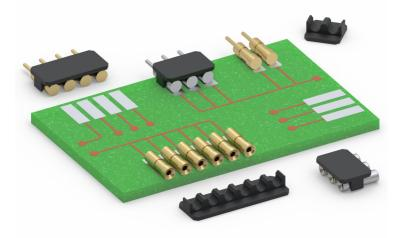
Mill-Max is proud to present new Horizontal SMT (HSMT) headers and sockets ideally suited for low profile parallel board-to-board or board-to-component mating. The removable plastic cap provides the convenience of a traditional connector and once removed delivers an interconnect system with a minimal surface mount profile.
