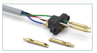
Mill-Max is proud to announce a new addition to its spring-loaded pin selection with the introduction of the 0973-0-15-20-77-14-11-0. This new offering has a solder cup designed to accept up to 20 AWG wire, has a maximum stroke of .080" (2,03 mm) and can be used at a minimum spacing of .100" (2,54 mm).
