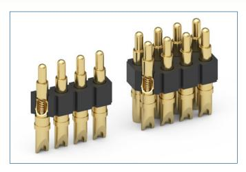
Mill-Max is expanding our solder cup, spring loaded connector series with the introduction of new versions delivering over 60% more stroke than the existing series. The single row 824-22-0XX-00-005000 and double row 826-22-0XX-00-005000 provide a mid-stoke of .045" (1,14 mm) with a maximum stroke of 090" (2,29 mm). The longer stroke helps compensate for tolerance stack-ups in assemblies and provides greater flexibility for unpredictable motion due to shock and vibration.
