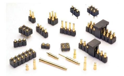
Mill-Max SLCs are button type contacts interconnecting two parallel conductive surfaces inside an electronic device or instrument. The stroking movement of the spring pin piston accommodates uneven, non-parallel conditions due to mechanical tolerances in the assembly.
