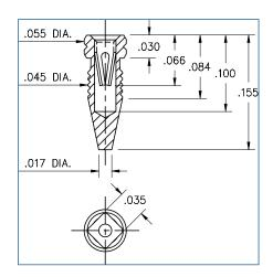
Mill-Max is pleased to announce the development of a unique, low-profile, compliant body socket receptacle capable of press-fitting in FR-4 mounting holes between .041" - .044" (1,04mm - 1,12mm) in diameter.
