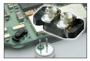
• Microphones must be hand soldered or socketed because the Mylar diaphragm inside the microphone would melt if it were reflow soldered directly to the circuit board. A socket eliminates the expense of hand soldering.
