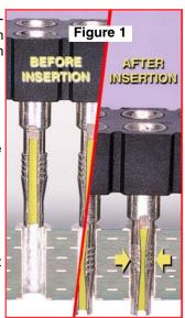
Compliant tail press-fit pins are solving many packaging problems for design engineers, especially in use with multi-layer backplanes which are typically too thick for soldering. These multi-layer backplanes, or motherboards, are extremely intricate in their construction and can be easily damaged during board assembly.
