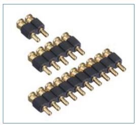
Utilizing Mill-Max's state-of-the-art, high quality precision-machining technology, these durable spring pins are designed to assure a 1 million cycle life minimum. Rated at 2A continuous (3A peak), the pins are plated  $20\mu''$  gold over nickel on the piston and base, with  $10\mu''$  gold over nickel plating on the beryllium copper internal spring.
