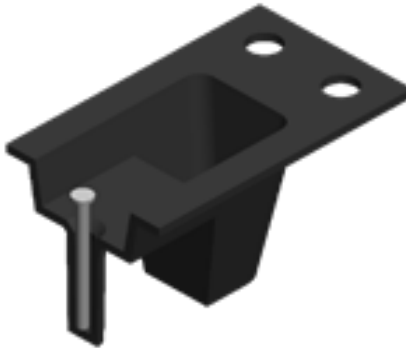
Nail Head Pins in "Head Up" Orientation
