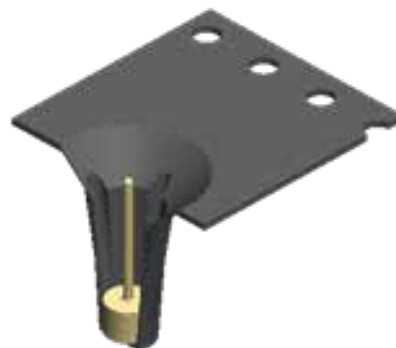
Nail Head Pins in "Head Down" Orientation
