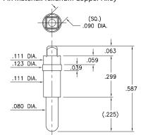
Recommended drilled hole sizes are prior to plating of the PCB and based on typical copper deposition of .5 - 1 oz. This results in a reduction of hole size by approximately .0015" - .003". Depending on surface plating, typical finished hole sizes are .003" - .005" smaller than drilled hole sizes. The finished hole size tolerance for press-fit applications should be specified as +/- .002"
